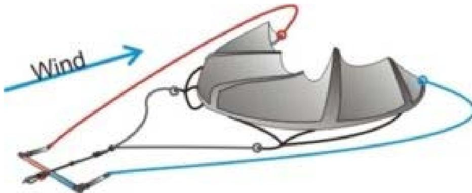
*Kite with lines correctly installed*
